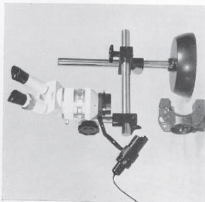
Fig. 5 M5 stereomicroscope with 0.5 x additional objective on swinging arm stand
