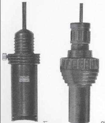
the microscope and the frosted glass insert should be replaced by clear glass. The mains lamp is switched on and off by rotating the collar round the bulb socket; the low voltage lamp is operated via the transmitter.
